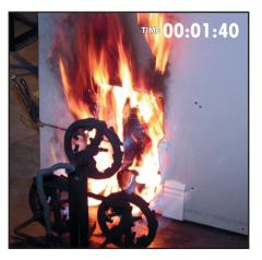
Time elapsed for fire to penetrate wall cavity
